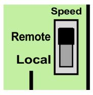
With switch SW2 set to the "REMOTE" position, the local control adjust potentiometer will be disabled. Fan speed will then be controlled by a variable 0-10v dc input signal applied across the appropriate terminals of the remote speed input:
