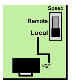
Fan speed will be controlled by the position of the Local Control adjustment potentiometer. The precise set-point can be attained by measuring the dc voltage across the adjacent test terminals (or alternatively across the "0v" and "CTRL" terminals of the Fan Connections).
