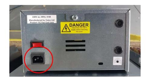
Fig 5.6c: Power supply connection point
