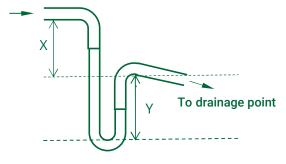
**Fig 5.3a:** Heat exchanger coil drain trap
