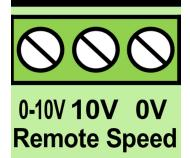
The "10v" terminal does not need to be connected, however it may be used if required to provide a 10v dc reference signal for use with a potentiometer device.
