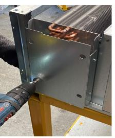
Fig 8.3a: Coil end protection plate
