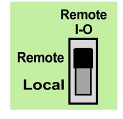
A volt-free contact should then be connected across the remote on/off input terminals. The fans will be enabled and will run at the set speed when the contacts are closed.
