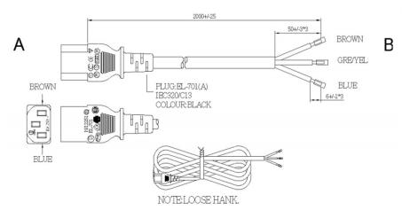
Fig 5.6c: Standard Optional Kettle Lead
