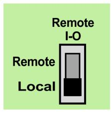
Where the operation of the fans is to be controlled via an enable signal, switch SW1 should be set to the "REMOTE" position as shown below:
